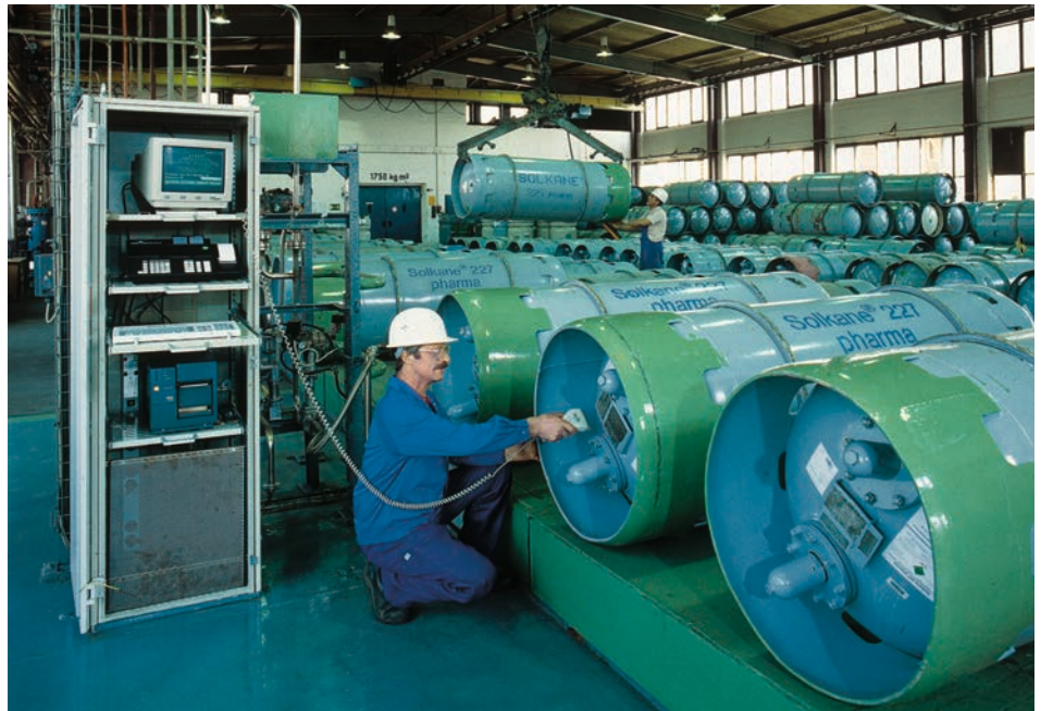
Electronic bar code scanning of SOLKANE™ 227pharma one tonne cylinders for identification and traceability.
