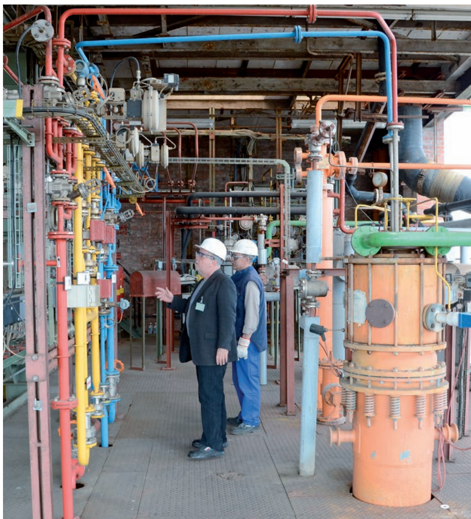
Reprocessing of HF and HCl from CFCs, HCFCs and HFCs by thermal decomposition.
