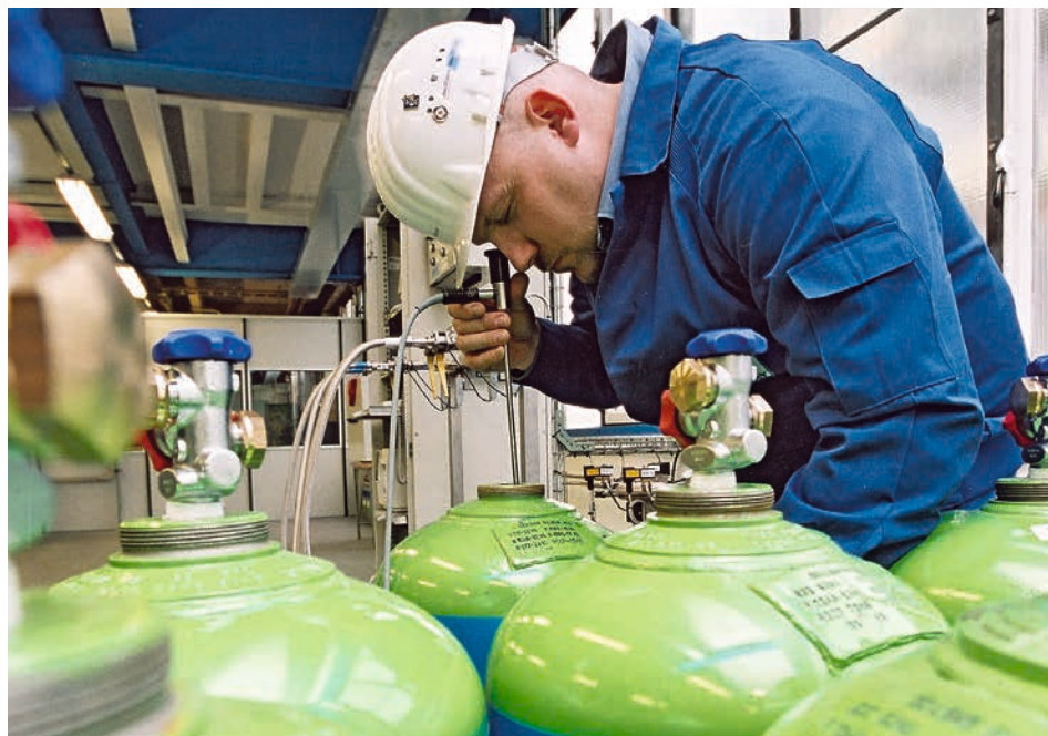
Visual inspection of dedicated pharma cylinders as part of Daikin's quality control.
