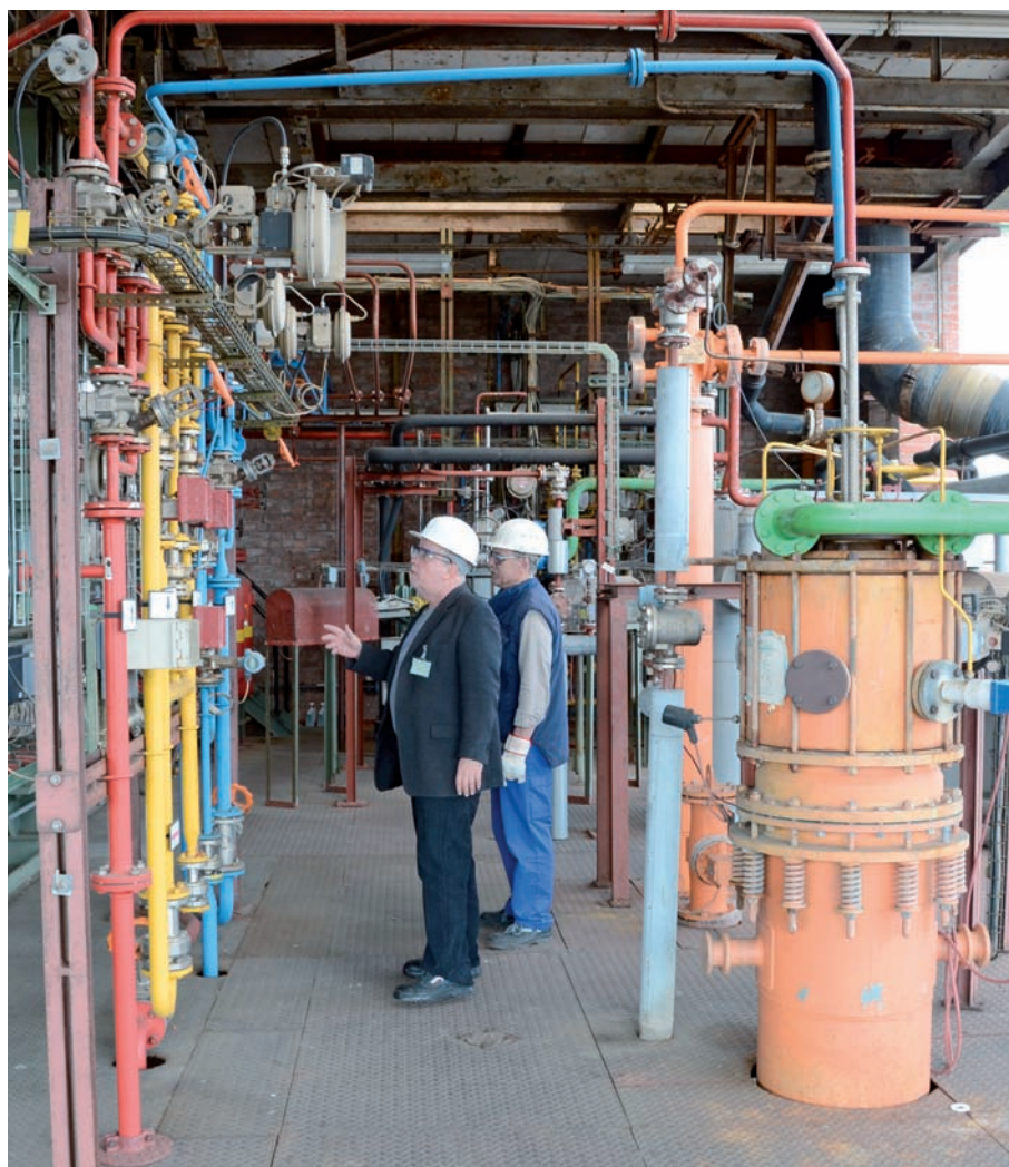
Fig. 31: Reprocessing of HF and HCl from CFCs, HCFCs and HFCs by thermal decomposition
