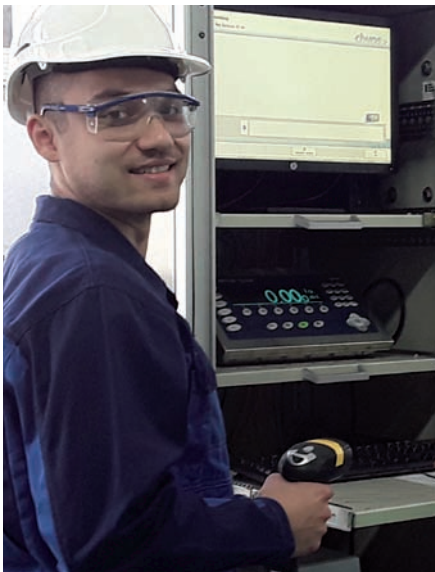
Fig. 5: Electronic bar code scanning of SOLKANE™ 134a pharma cylinders for identification and traceability
