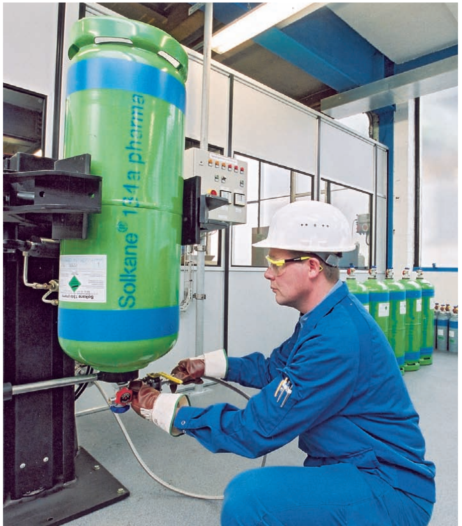
Fig. 3: Cleaning cylinders prior to use for SOLKANE™ 134a pharma according to Standard Operating Procedures (SOPs) in the area designated for SOLKANE™ pharma products only
