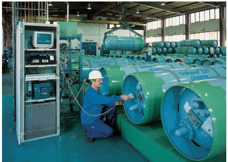
Fig. 9: Electronic bar code scanning of SOLKANE™ 227 pharma one tonne cylinders for identification and traceability
