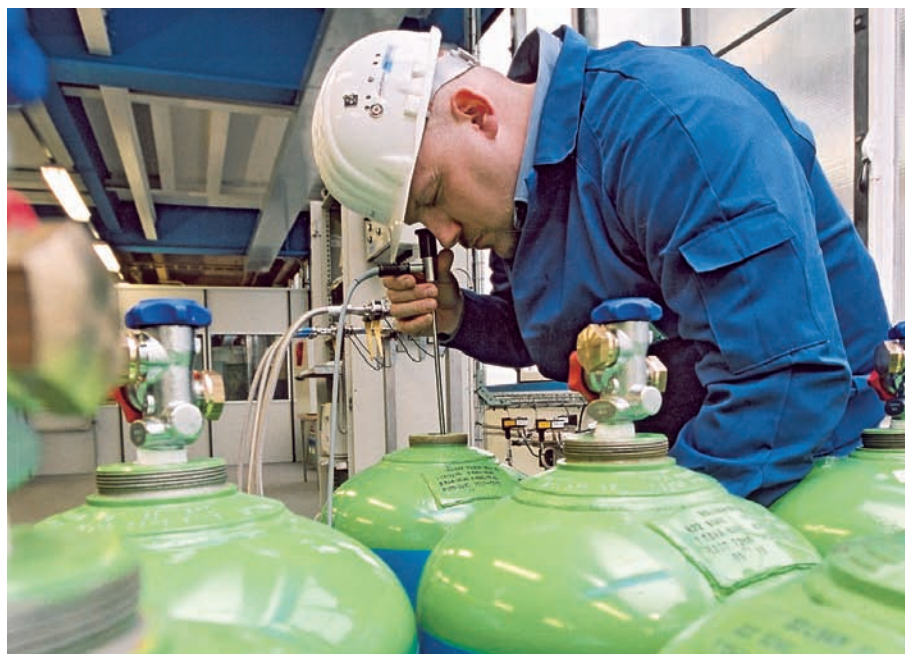
Fig. 7: Visual inspection of dedicated SOLKANE™ 134a pharma cylinders as part of Daikin's quality control
