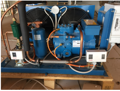
Fig.2: Compressor / condenser racks
