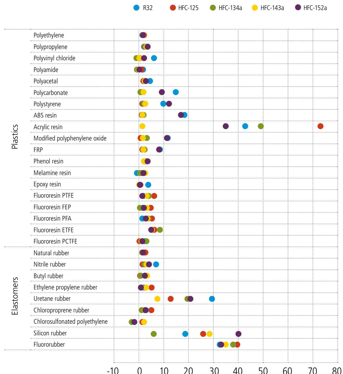
Measurement conditions: Immersed in refrigerant at 50°C for 2 weeks.
